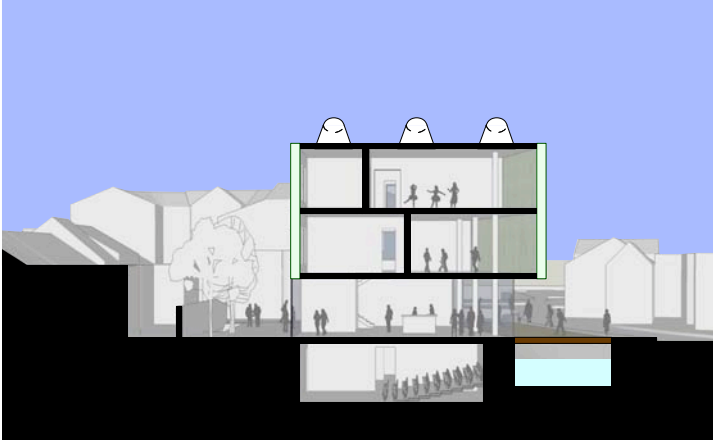
Diagram 7. Section through building showing performance area at basement level. Foyer is open to both courtyard and boardwalk bridge creating strong urban relationships.
